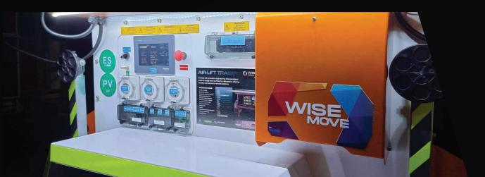
Inside its exterior lies a robust energy storage system, capable of storing up to 15.36kwHr and delivering an output of 6000VA. Whether It's for powering remote construction sites, supporting disaster relief efforts, or enabling off-grid operations, this trailer ensures reliable energy wherever it's needed most.
